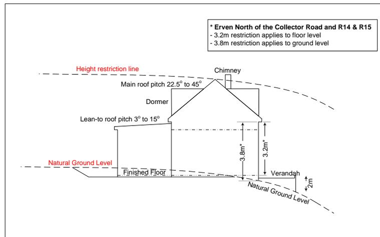
3.2.4 All dormer windows are to conform to the window proportions described in this manual and are to be clearly subservient to the major roof forms, (i.e. less than 50% in plan and elevational area). The design approval of these is at the DRC's discretion.
